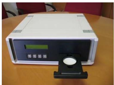
Magee Scientific Model OT21 Optical Transmissometer.
