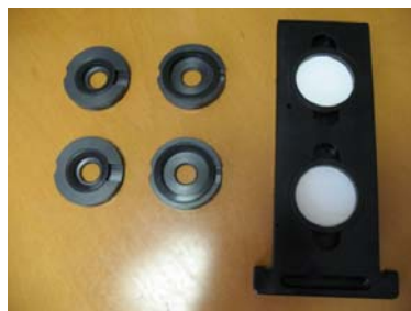
Filter slide tray and adapters for 25, 37, and 47-mm diameter samples.
