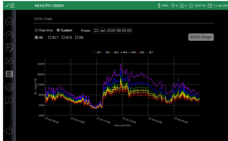
Figure 1: Data from all 7 wavelengths shown in a single chart.
