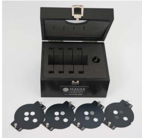
**Figure 5:** Optical Validation Kit consisting of traceable standard Neutral Density Optical Filters, which are inserted into the AE33 optical path to determine the reproducibility of the relationship between LED optical source intensity and detector response.
